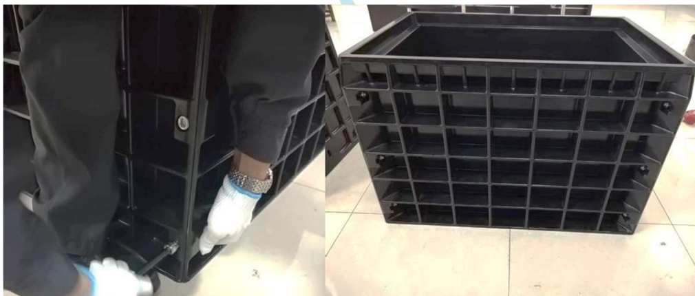
3.2.6 Secure 12 pcs bolts on the panels
