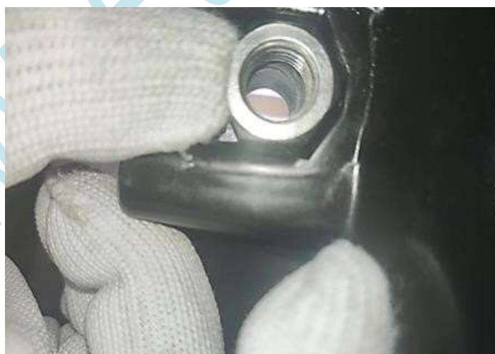
3.2.3 Place the inner hexagon nut into the fixing slot
