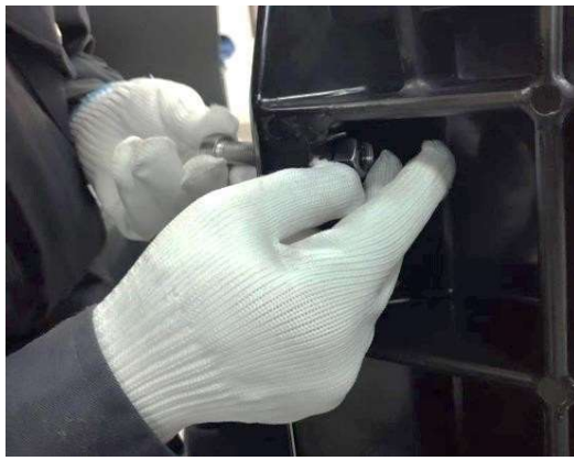
3.2.4 Place the inner hexagon bolt into the nut
